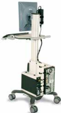
Cable management keeps cables hidden yet easily accessible.
